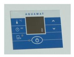
The preparation for the work consists in setting of the needed time and temperature. The adjustments are done using the selection buttons - button  $^{\circ}$  and button  $^{\circ}$ .
