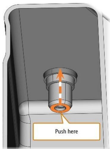
FIG. 86 – PUSHING THE COUPLING OUT OF THE TANK
