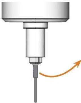
FIG. 58 – REMOVING THE TOOL FROM THE COLLET CHUCK
