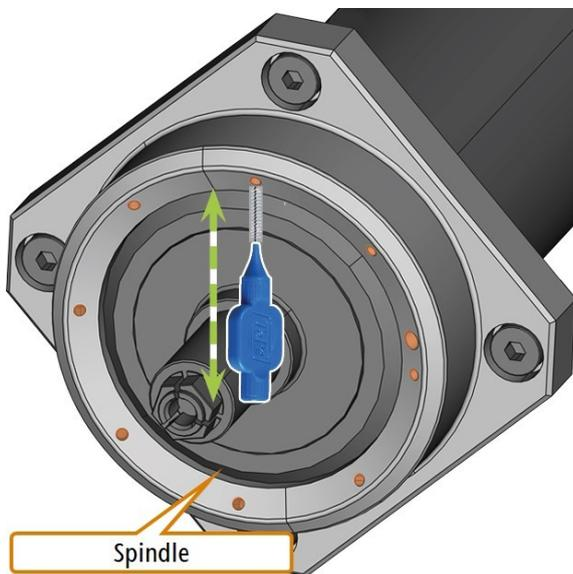
FIG. 78 – CLEANING THE NOZZLE PLATE; NOZZLES MARKED ORANGE
