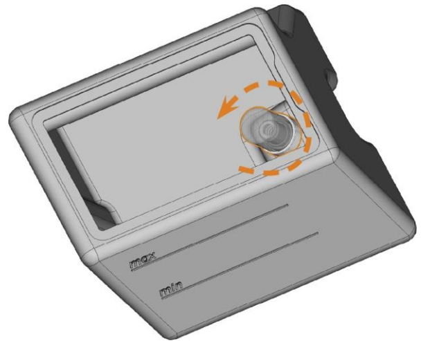
FIG. 90 – UNSCREWING THE FILTER IN THE COOLING LIQUID TANK
