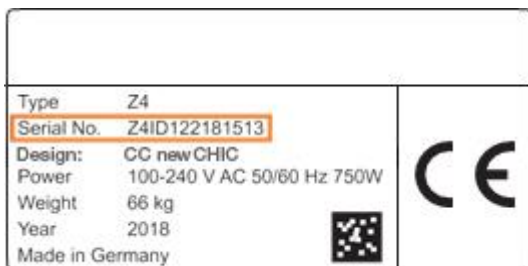
FIG. 9 – SERIAL NUMBER ON THE IDENTIFICATION PLATE (MARKED ORANGE)
