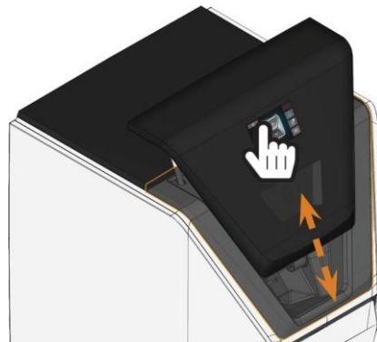
FIG. 30 – OPENING & CLOSING THE WORKING CHAMBER DOOR
