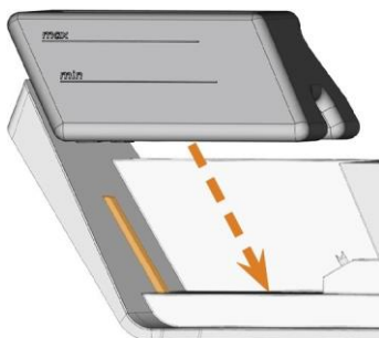
FIG. 39 – INSERTING THE COOLING LIQUID TANK INTO THE DRAWER (GUIDE RAIL COLORED ORANGE)
