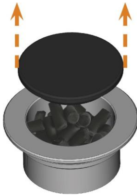
FIG. 84 – OPENING THE CARBON FILTER
