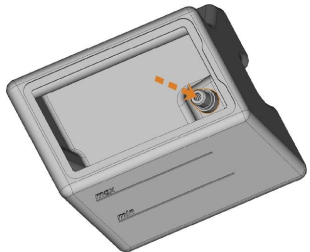
FIG. 91 – PUSHING THE COUPLING OUT OF THE TANK
