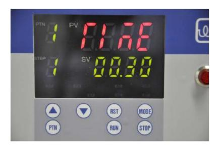
Use the ★★ keys to set the time in which the temperature is to rise to the set level in the first step (SV Display).
