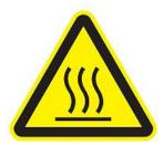
When the oven is hot, close the door immediately after removing the cuvette. The oven may not be forcefully cooled by opening the door as this will result in additional heating of the exterior surface. Furthermore, when the door is open, temperature in the oven interior cannot be reliably estimated which in turn could lead to burns.
